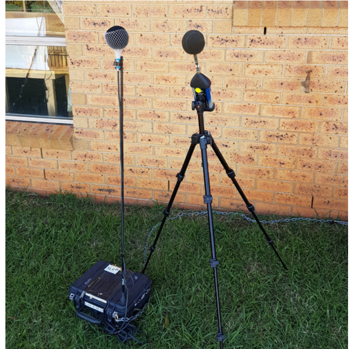
Above: Example of a noise monitoring device placed near the most exposed façade of a residential building.
